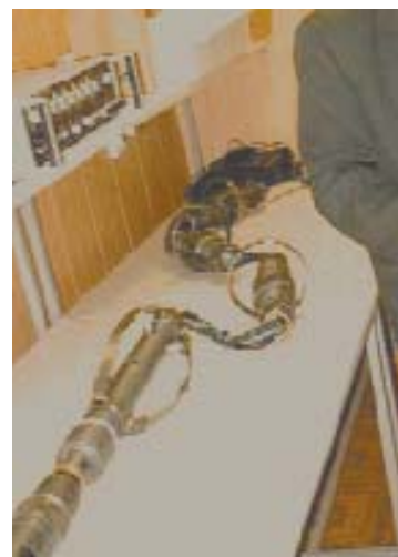
Figure 1: Through-casing resistivity equipment in the laboratory. In the foreground one can see the electronics cartridge. The background depicts the measurement electrodes.
