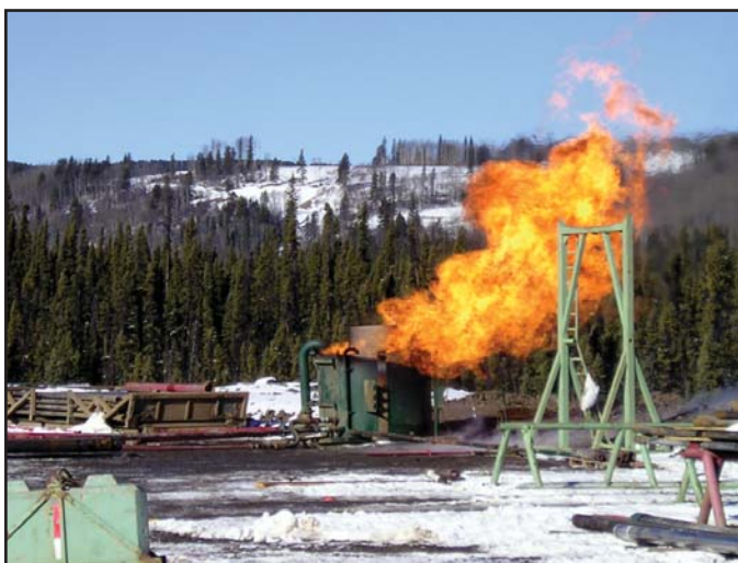
Flare from a Bluesky gas kick. Photo courtesy of Running Horse Resources.
