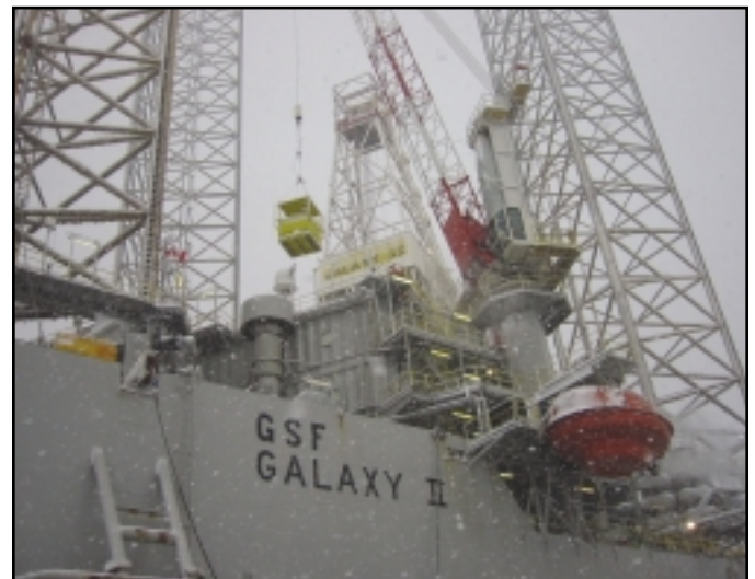
Global Santa-Fe's Galaxy II Jack-up Platform in the Halifax harbor, January 2004. Two of the jack-up towers (foreground) and in the drilling rig (center background) are visible. The platform can operate in a maximum water depth of 110m.
