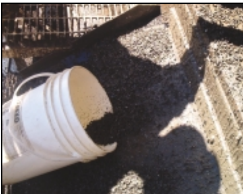
Photo 2: Bucket used to catch sample from shale shaker. Courtesy G. Gorman
