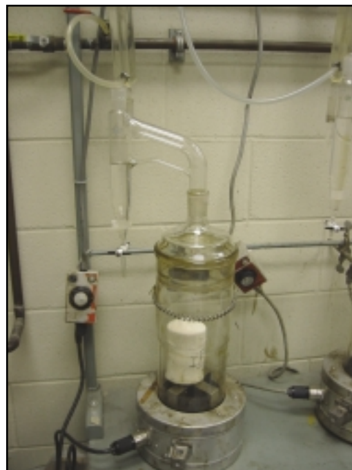
Dean Stark apparatus used to determine the water content of a core sample.
