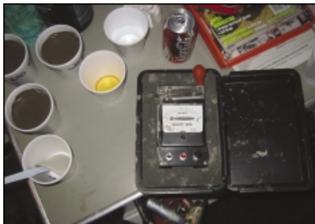
The resistivity meter used to make R_{mf} , R_m and R_{mc} measurements in a logging truck. Note the cup of amber colored filtrate.
