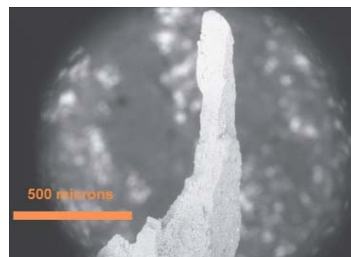
Figure 14. A black shale sample ready for nanoCT scan. Scale at 500 \mu\text{m} .
