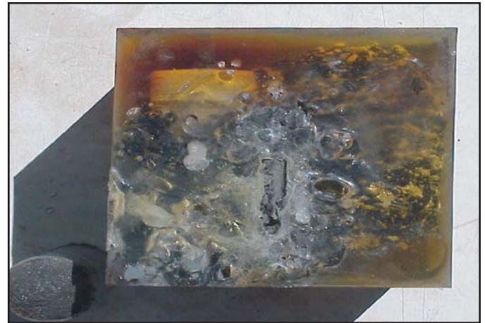
Figure 1 – Coal Seam Sample Cast in Resin for Drilling
