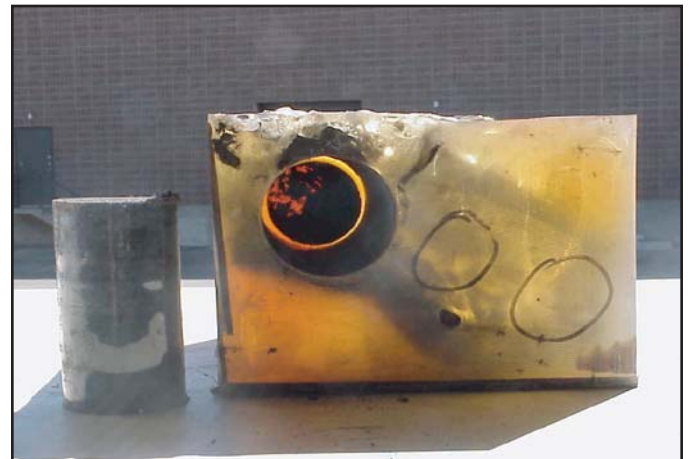
Figure 2 – Illustration of Drilled Intact Coal Plug with Fractures and Cleats Preserved for Mounting for Formation Damage Testing
