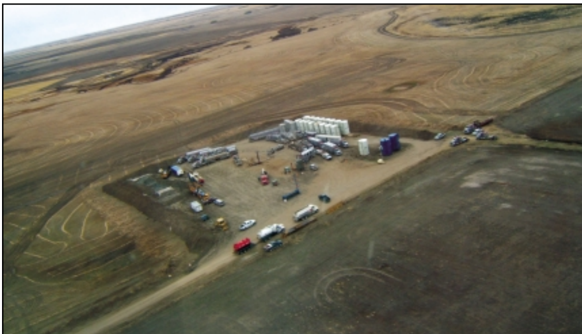
Frac operations for a Bakken horizontal well in SE Saskatchewan. In the photo can be seen the 4 pumpers, 3 nitrogen trucks, command shacks and the eighteen 400 barrel tanks required to complete the operation. A total of 240 tonnes of sand was pumped in this multi-stage frac completion. Photo Courtesy Ben Urlwin.
