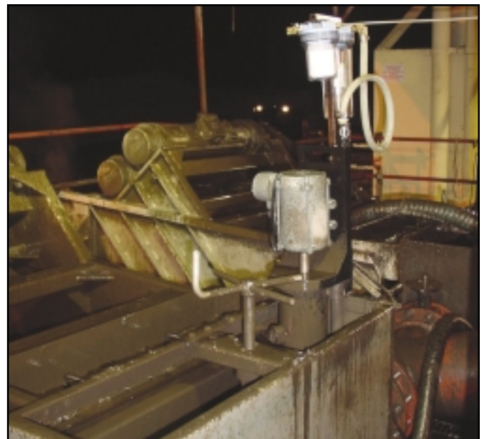
A working gas trap and dryer assembly fastened to the 'possum belly' of the shaker.
