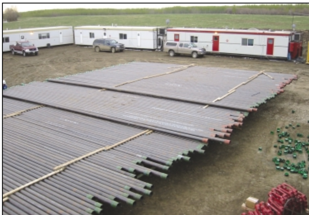
Removing thread protectors from production casing in preparation for drifting and quality inspection.
