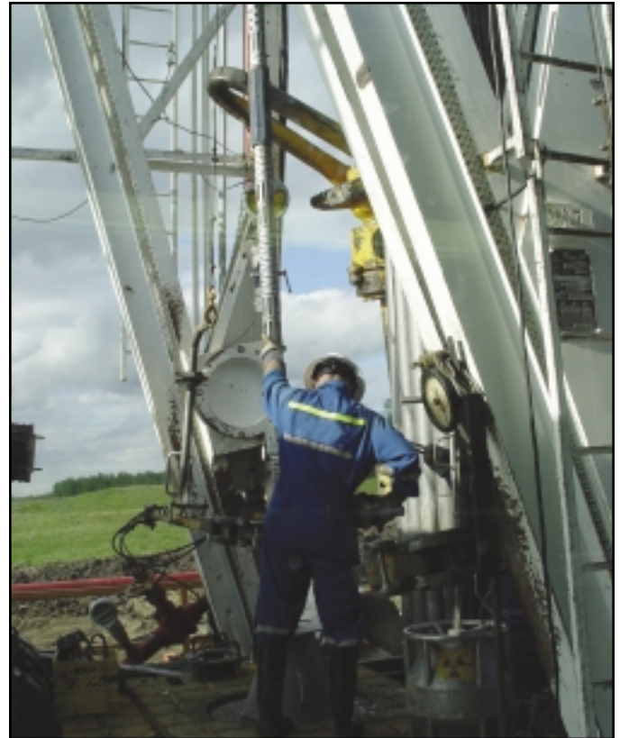
Rigging up a sonic tool in the Hoadley area, AB. Photo courtesy Dave Kelly
